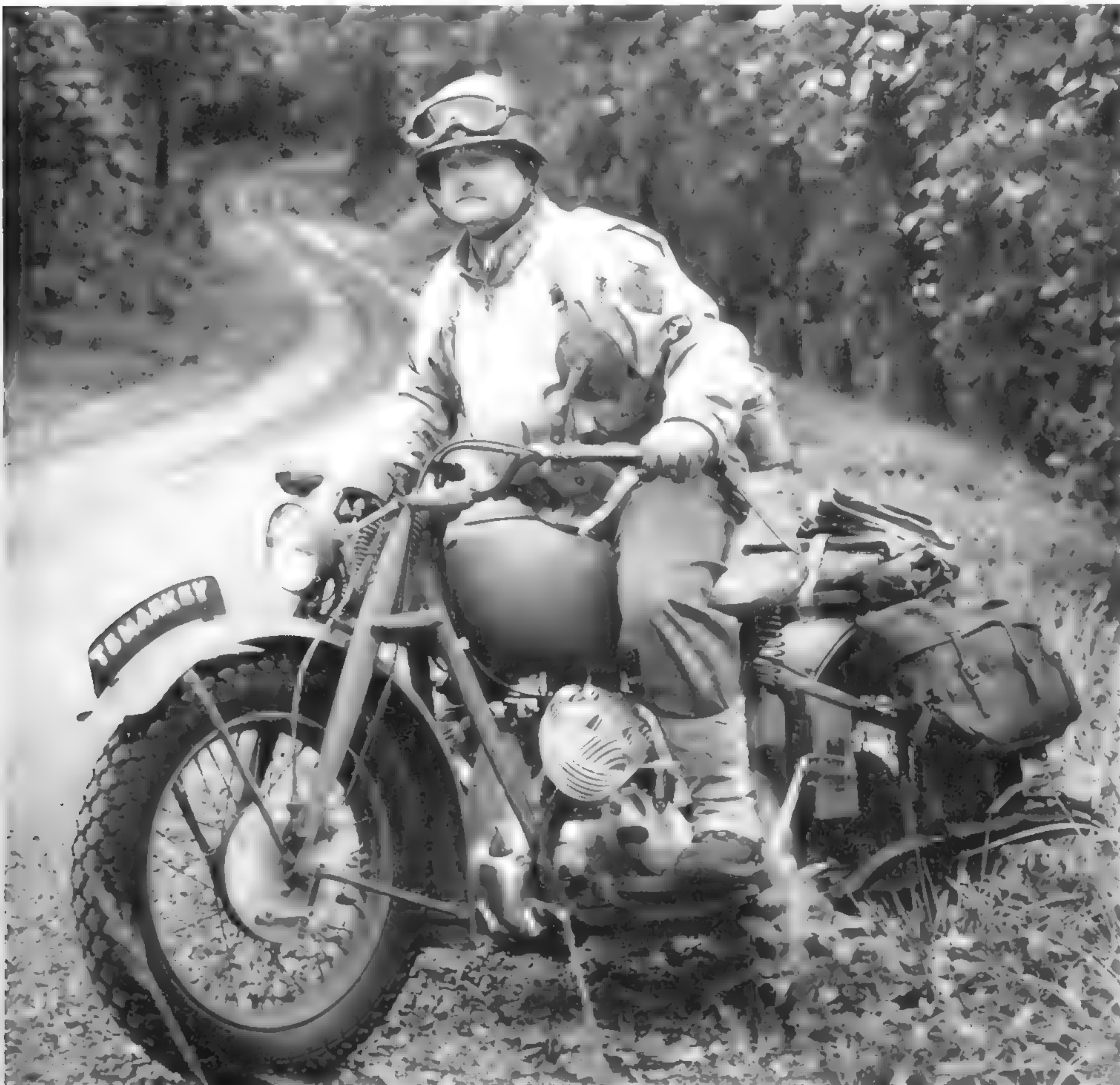
Among the most sought-after Indian military motorcycles is the shaft-driven model 841. The shaft drives were developed based on the BMW R71 idea, and were intended for desert use. However, the widespread use of the Jeep precluded their deployment. Robin Markey is astride this beautifully restored example. Notice the cylinder heads protruding just ahead of his knees on either side. (Photo from the collection of Robin Markey and Bob's Indian Sales and Service)
